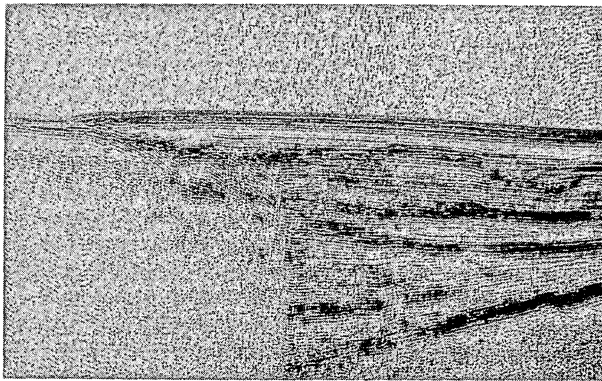
FIGURE 99[5].—Subbottom profile at fix 675 of section 4. Basement or volcanic rocks on left abut against sediments on right. A fault separates the contrasting subbottom structural features at depth, but is covered by overlying sediments at the sea floor.
