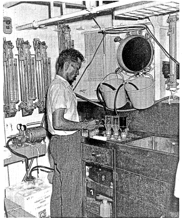
FIGURE 105[2].—Apparatus used for seston and pigment sample preparation in ship laboratory.
