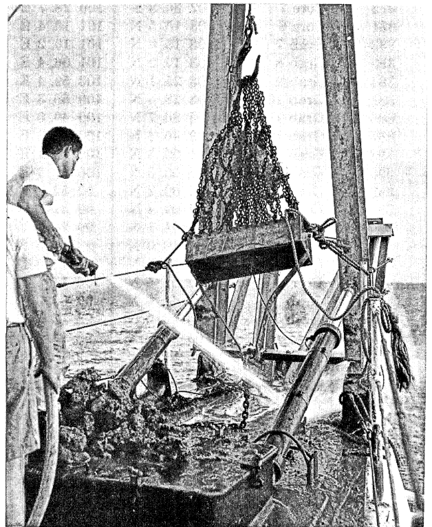
FIGURE 60.—Emptying contents of chain bag dredge.
